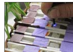
Fig. 1 Optode-based device for imaging pH gradients in the rhizosphere of Durum wheat seedlings. Upon excitation with light, the pH-responsive optode (white rectangle in contact with the roots in the rhizotron) delivers a fluorescent signal correlated with the pH value. P. Hinsinger, unpublished results.
